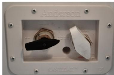
4. Set the compressor to 40 psi or less and turn it on. If no faucets are open, the compressor should reach 40 psi in a few seconds and stop running.
